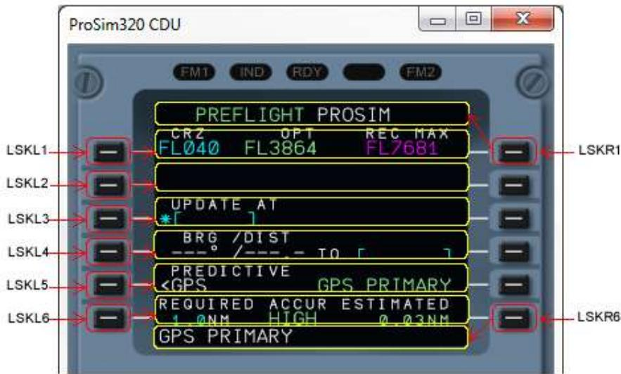
The first line (LSKR1) should be lighted in a yellow square box. Align the line by using the following commands:
